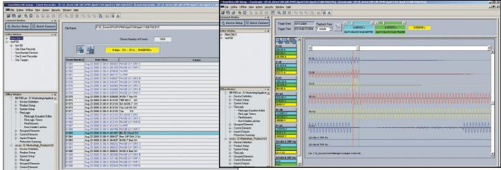
Record the operation of the internal F60 elements and external connected devices with 1ms time-stamped accuracy to identify the Sequence of Operation of station devices during faults and disturbances.
