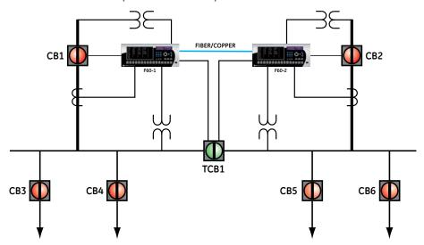
Auto-transfer schemes can be implemented using programmable FlexLogic. Wiring between relays can be eliminated using peer-to-peer communication.
