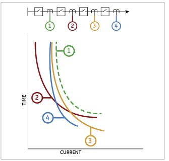
Custom FlexCurves can be constructed to coordinate with other upstream and downstream protection devices.
