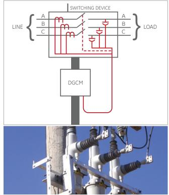
Detection functions and FlexLogic enable the Multilin DGCM to be used for most pole top applications.
