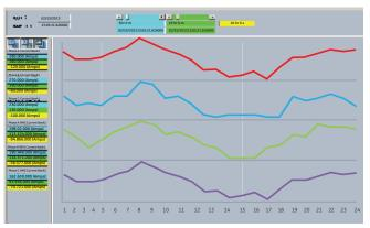
The Multilin DGCM data logger helps in better understanding the analog channel behavior, by sampling at a selectable time interval rate of 1 to 60 minutes.
