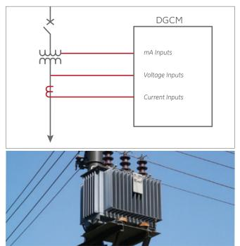
Transformer monitoring with the Multilin DGCM enables overload identification, which is key for load planning and asset management.
