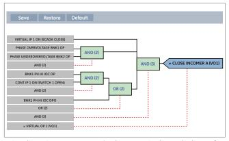
Using FlexLogic, customers can develop customized control schemes for multiple applications.
