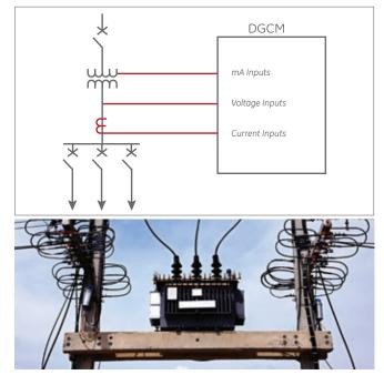
Volt/VAr control schemes are better optimized using the Multilin DGCM, as changes in voltage (real-time) are reported almost immediately (unsolicited messaging) over most utility protocols.
