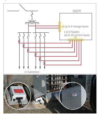
Monitoring at key LV consumer substations with the Multilin DGCM can help in faster fault isolation and energy theft detection.
