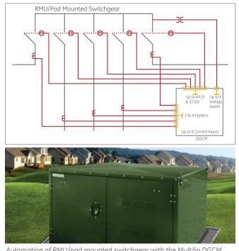
Automation of RMU/pad mounted switchgear with the Multilin DGCM improves grid reliability by reducing outage time.
