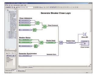
The internal operation of the G60 elements, logic, and outputs can be monitored in real-time to simplify commissioning and troubleshooting procedures.
