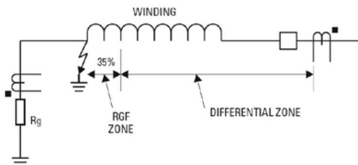
Faults close to the neutral point of a wye-connected winding does not generate adequate fault current for elements to detect. Restricted ground fault protection provides sensitive ground fault detection for low-magnitude fault currents.
