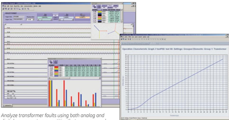
Analyze transformer faults using both analog and digital power system quantities that are measured and recorded up to a rate of 64 samples per cycle.
