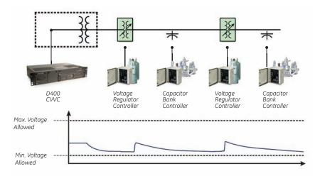
When integrated with an IVVC or CVVC system, Vol/VAR controllers provide regulated voltage levels with minimal fluctuations along the feeder segment, they ensure voltage is maintained within allowable limits, and they improve power factor which reduces line losses (VAR reduced).
