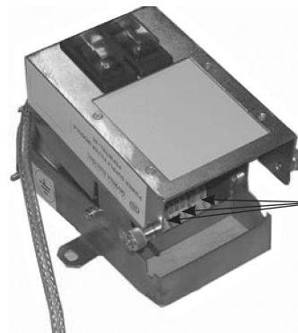
Figure 44 PSFM connectors XS1, XS4, XS5 (PSFM is open)
