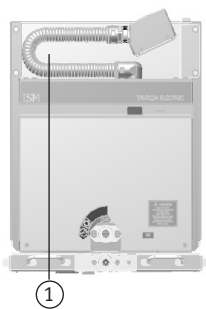
Figure 16 Labelling Draw-out unit
