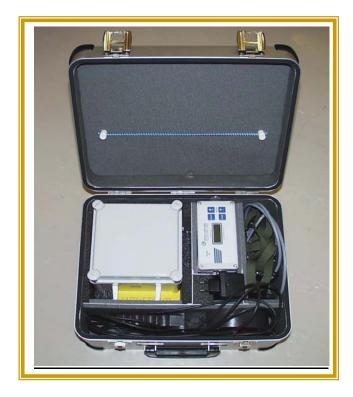
NCM-20 has two voltage clips by which the current is supplied into the capacitor bank. The voltage output is short-circuit proof.
